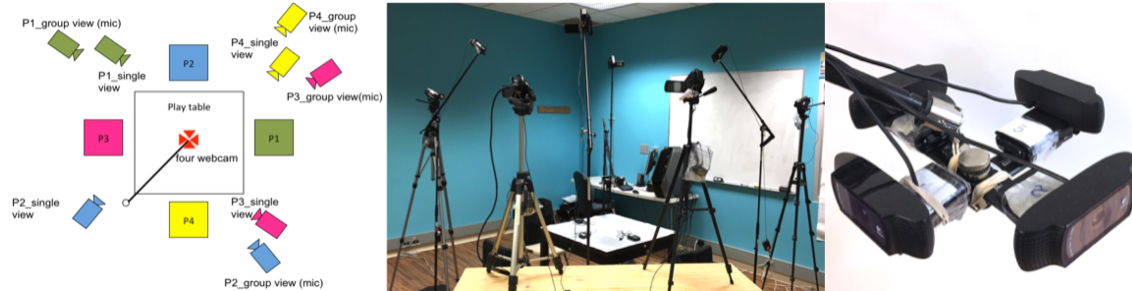
Fig. 4. In-lab study data collection apparatus. Left: illustration of the equipment arrangement; Middle: real equipment arrangement; Right: fixture of the four Webcam devices.
